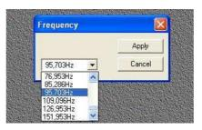
For EX controllers, the default choice for frequency setting is 95.7 kHz. If the display noise is high at this setting, you may try other frequencies to reduce the effects of noise on touch performance – 109 kHz and 76 kHz have been tested.
