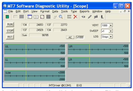
Scope is the most common tool for troubleshooting your touch system. This utility presents Format Raw corner data graphically as would a four channel digital oscilloscope.
